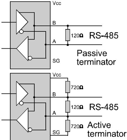
Both the RS-485 link ends should be terminated with the 100-120Ω resistors (so-called passive terminators), which are placed between A-B wires. These terminators are used for the converter impedance matching, they suppress the undesirable echo and they influence the transfer immunity against interference. Inserting the repeater into the metallic link terminates this link right on the A-B
