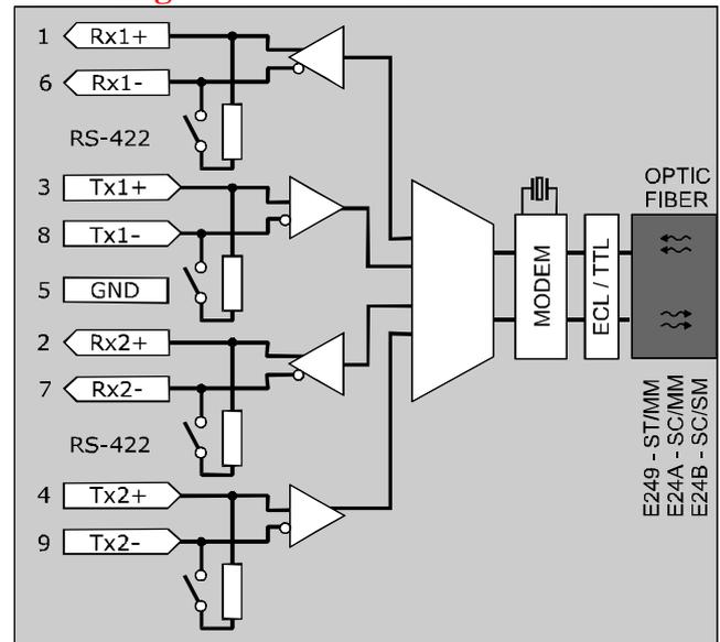
Modem ELO E24B is designed for singlemode fibers 9/125 μm. Its range is typically 15 km, optic connectors are SC type. For multimode cables 50/125 μm or 62.5/125 μm there are models ELO E24A with SC connectors and ELO E249 with ST ones.
