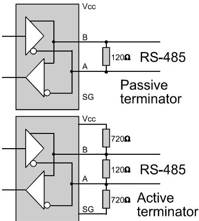
The RS-485 line should be terminated with the 100-120 Ω resistors on both ends placed between A - B conductors (so-called passive terminators). These terminators are used for the converter impedance matching, undesirable echo suppression and they influence transfer immunity against interference. There are also the active terminators beside the passive ones. Only one active terminator can be installed to one metallic section of the link and its role is as follows:
