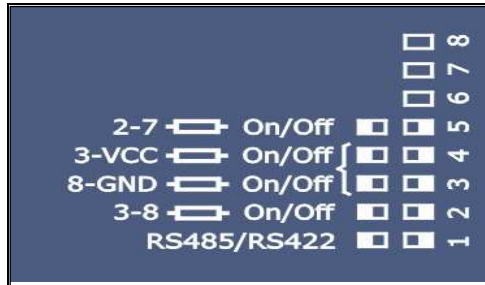
Pic. 1: DIP-switch description
